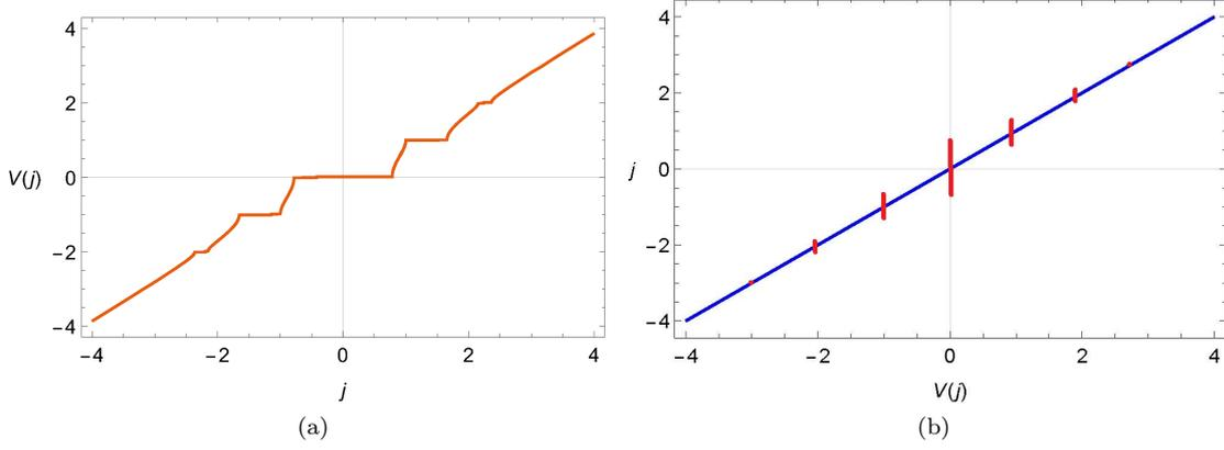
Fig. 4.2: Shapiro steps a); and Shapiro spikes b)
