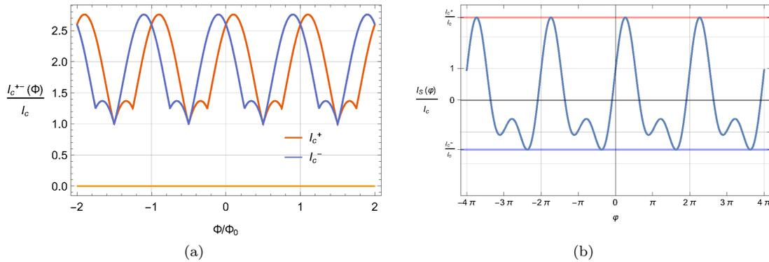
Fig. 1.2: (a) – critical current as function of the magnetic flux in case  $A = 1$ . (b) – Current-phase relation in case  $A = 1$ ,  $\Phi = 0.2\Phi_0$
