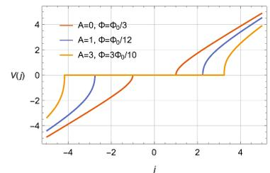
Fig. 2.1: Numeric result of the CVC in RSJ model under certain values of the parameters  $A$  and  $\Phi$
