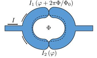
Fig. 1.1: Asymmetric Josephson junction based on two-contact SQUID. Asymmetry appear when  $\Phi \neq n\Phi_0, (n + 1/2)\Phi_0; n \in \mathbb{Z}$ .
