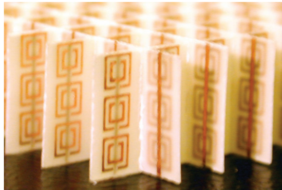
Fig. 1. Photograph of the left-handed metamaterial (LHM) sample. The LHM sample consists of square copper split ring resonators and copper wire strips on fiber glass circuit board material. The rings and wires are on opposite sides of the boards, and the boards have been cut and assembled into an interlocking lattice.
