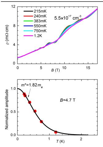
FIG. 4. Top: The Shubnikov–de Haas effect is visible in the magnetoresistance of the lowest doped  $SrTiO_3$  sample. Bottom: The effective mass obtained from the resistivity data is close to the one obtained by the analysis of the Nernst data.
