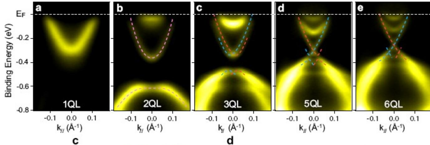
$$E_{\pm}(k_{\parallel}) = E_0 - Dk_{\parallel}^2 \pm \sqrt{(v_F \hbar k_{\parallel})^2 + \left(\frac{\Delta}{2} - Bk_{\parallel}^2\right)^2}$$
