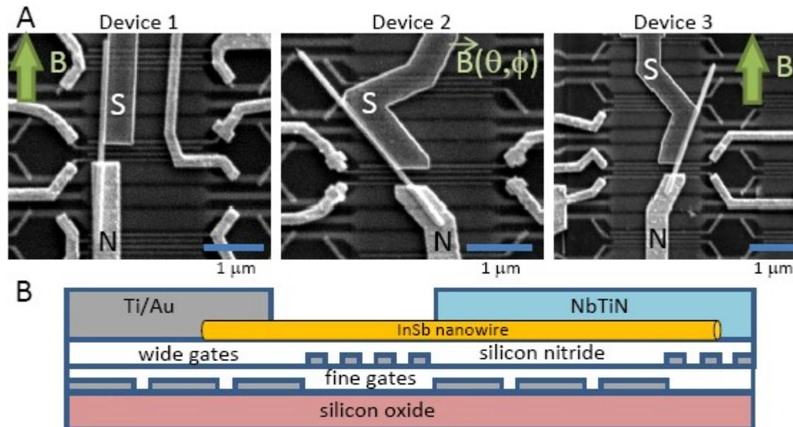
**A**, SEM images of three N-NW-S (Normal-Nanowire-Superconductor) devices in which the main findings of this paper are reproduced. Field directions are indicated with arrows. Device 2 was measured in a 3-axis vector magnet. Devices are fabricated simultaneously. Nanowire diameters are  $110 \pm 10$  nm (devices 1 and 3) and  $100 \pm 10$  nm (device 2). **B**, Schematic of a device cross-section.
