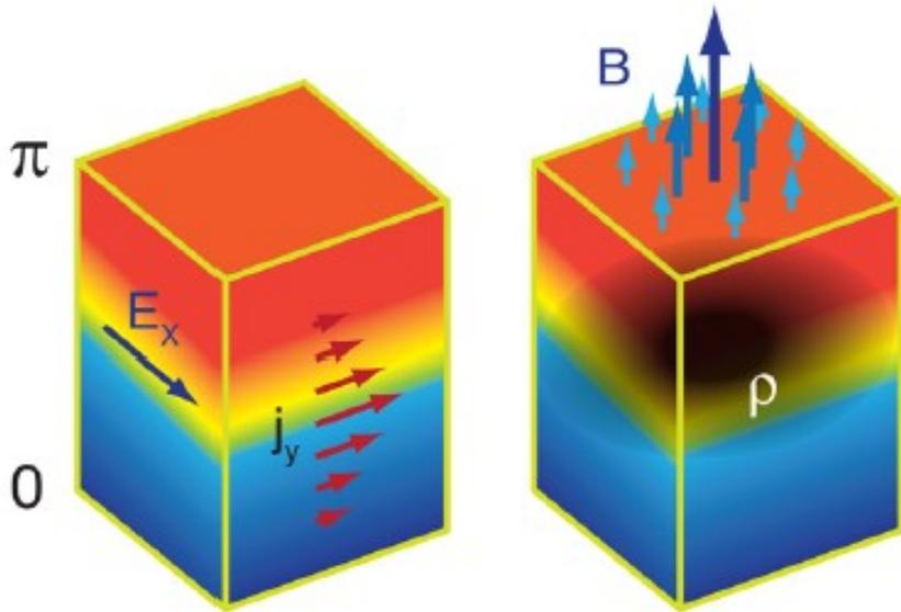
A magnetic field applied perpendicular to the same interface introduces  $(n + 1/2)$  electrons for each flux quantum of applied field. The shaded region corresponds to the charge density,  $\rho$ , of the electrons, which mainly concentrates around the boundary between the two insulators and is largest where the magnetic field is strongest. (Illustration: Alan Stonebraker/[stonebrakerdesignworks.com](http://stonebrakerdesignworks.com))
